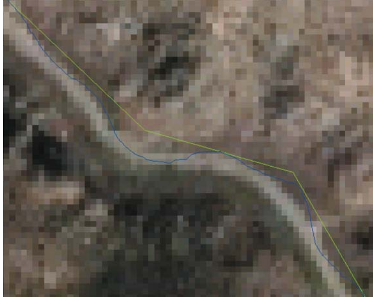
Fig. 7.27 Results from the second flight through Goshen Canyon. Flight test results show the planned path (green) and the actual path (blue). The planned path was intentionally biased to the east forcing the MAV to offset from its planned path to center itself through the canyon.
