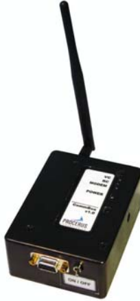
Fig. 7.5. Communication box connected to the laptop. The communication box contains a 900 MHz transceiver, a GPS unit, and an interface to an RC transmitter which can be used as a stand-by fail-safe mechanism to facilitate safe operations. Figure courtesy of Procerus Technologies.
