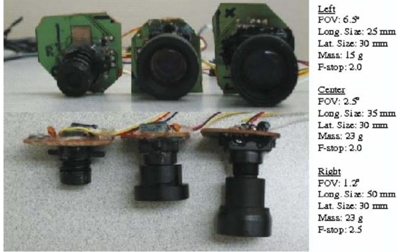
Fig. 7.6. Optic flow sensors with three different lens configurations: 1.2, 2.5, and 6.5 degree field-of-view. The optic flow sensors are constructed by attaching a lens to an optical mouse chip.
