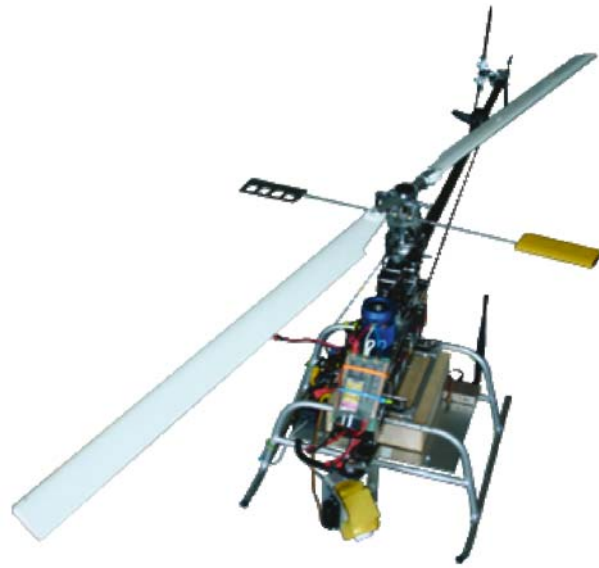
Fig. 4.1. Small helicopter with a custom-made controller and pan-tilt camera.
