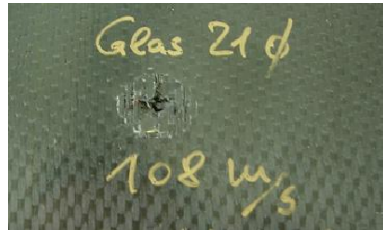
Fig. 19. Damage on upper skin and core.
