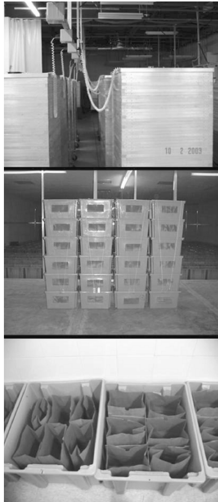
Figure 6. (upper) Mediterranean fruit fly emergence towers (Worley system), (middle) plastic adult release containers (PARC), and (lower) PARC boxes showing the pupae holding paper bags (middle and lower photo from F. Moscoso, reproduced with permission).
