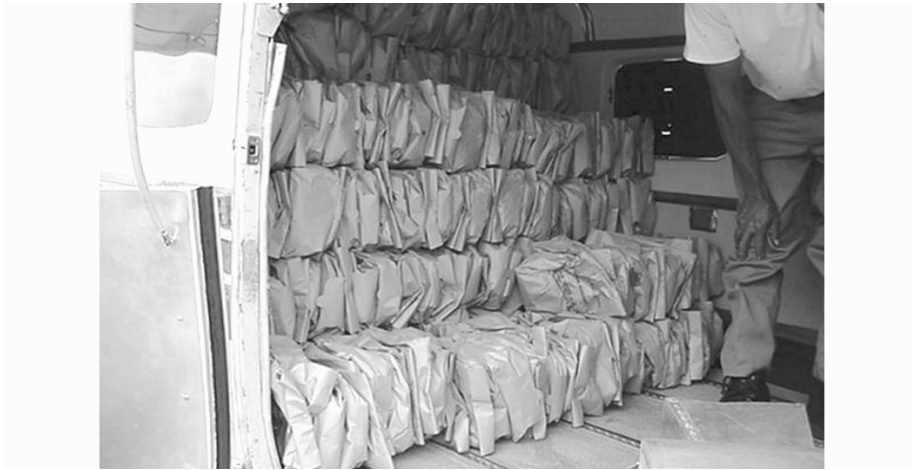
Figure 1. Paper bags stacked in the aircraft cabin prior to release through a chute constitutes the paper bag delivery system.
