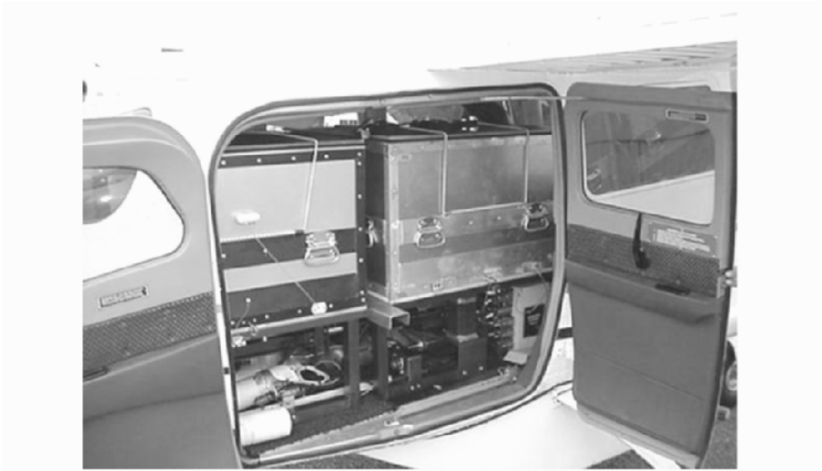
Figure 4. Second generation chilled adult release system installed inside a Cessna 206 aircraft.
