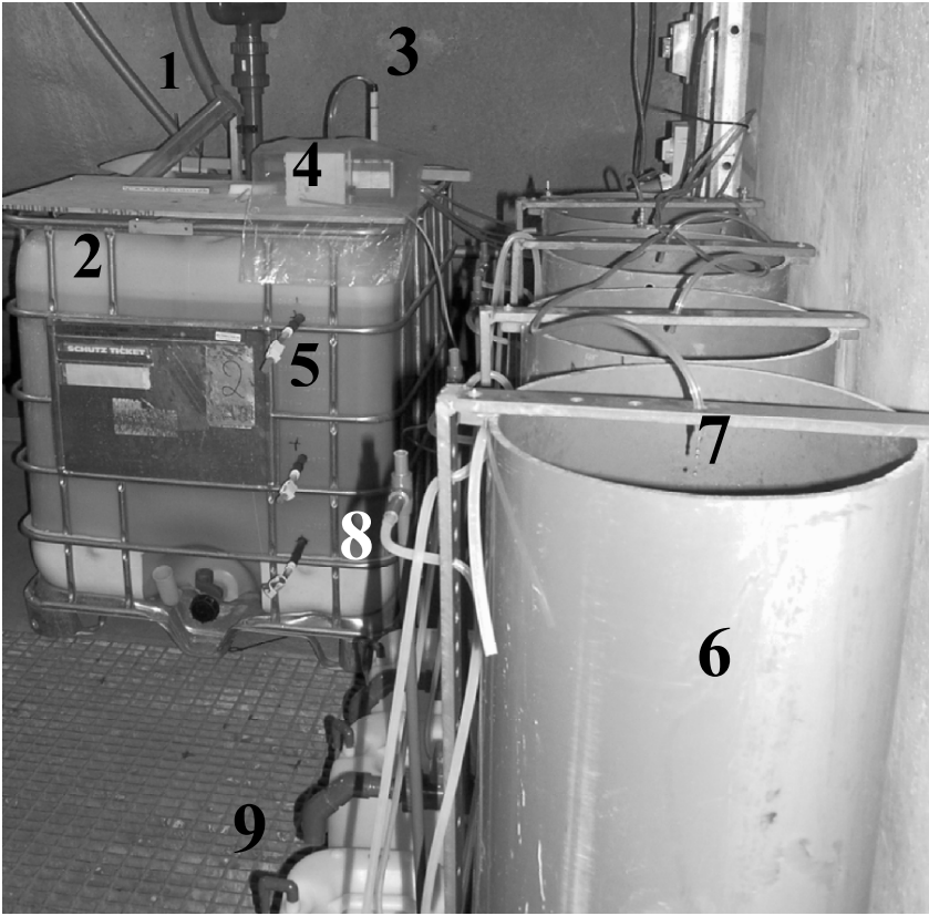
Fig. 1. Experimental set-up: inflow (1), tank (2), level control discharge to columns, peristaltic pump (4), sampling ports (5), column (6), discharge filter (7), level control filter (8), sampling vessel for filtrated water (9)
