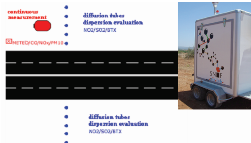
Fig. 2. Project of installation of the measuring equipment and Snif Lab
