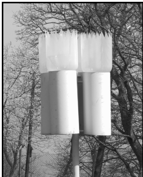
Fig. 3. Bulk precipitation collector
