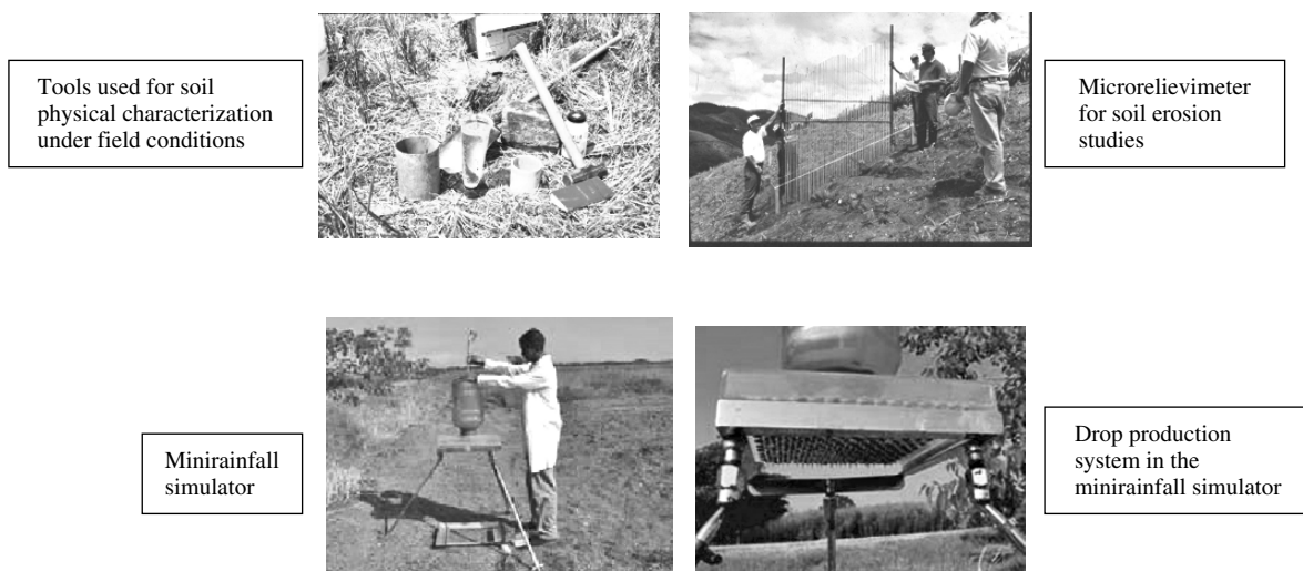
Figure 12. Field tools developed by CIAT to assess soil degradation in hillside areas.
