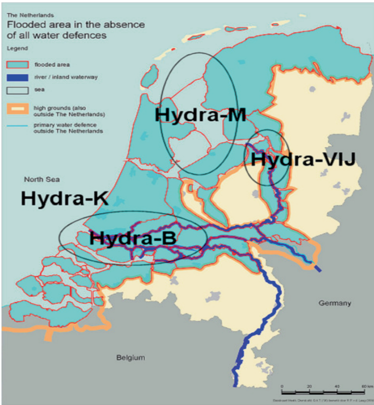
Figure 1. The areas in which Hydra-models can be applied shown on a flood vulnerability map
