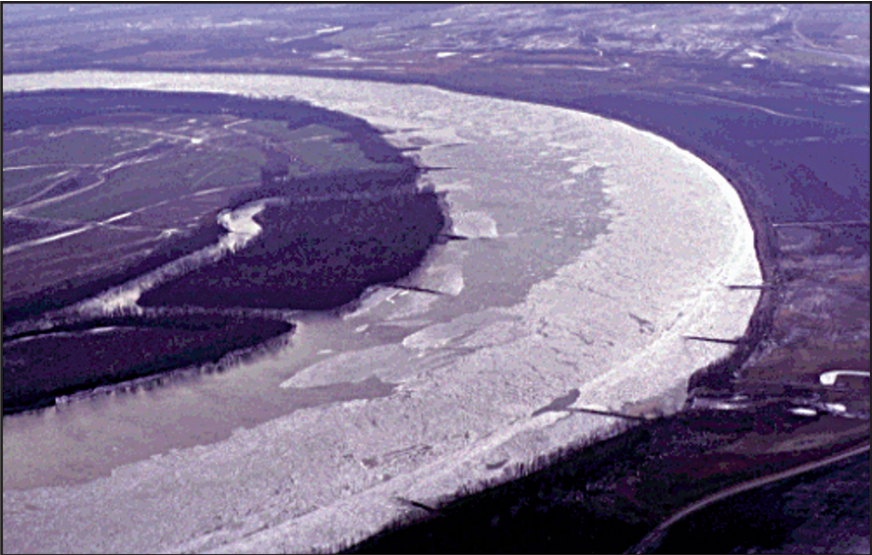
Figure 6. An ice run (of frazil slush) along the middle Mississippi River below St Louis poses an obstacle to navigation and commerce (Photo courtesy of Andy Tuthil of U.S. CRREL)
