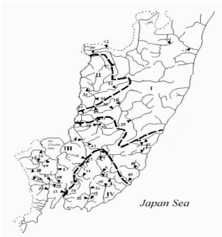
Figure 1. Division into districts of the territory of Primorski Krai according to the condition of uniformity of variation coefficient of maximal river runoff
