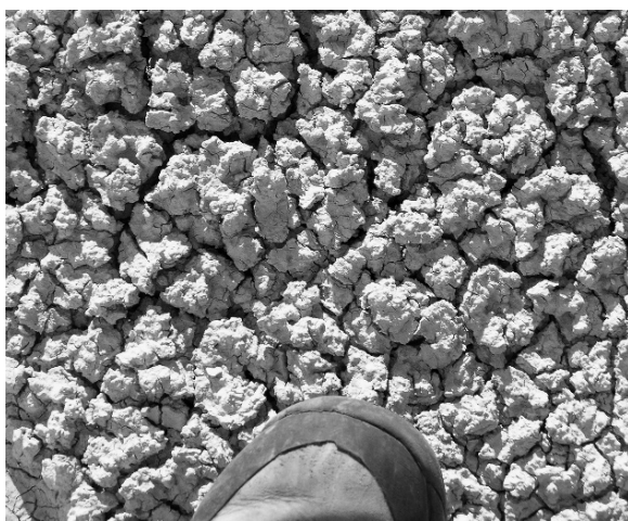
Fig. 10.4 Popcorn surface crust on Morrison Formation shale. Clays in these badlands are dominated by Smectite (Montmorillonite) clays with high shrink-swell potential (photo by A. Howard)
