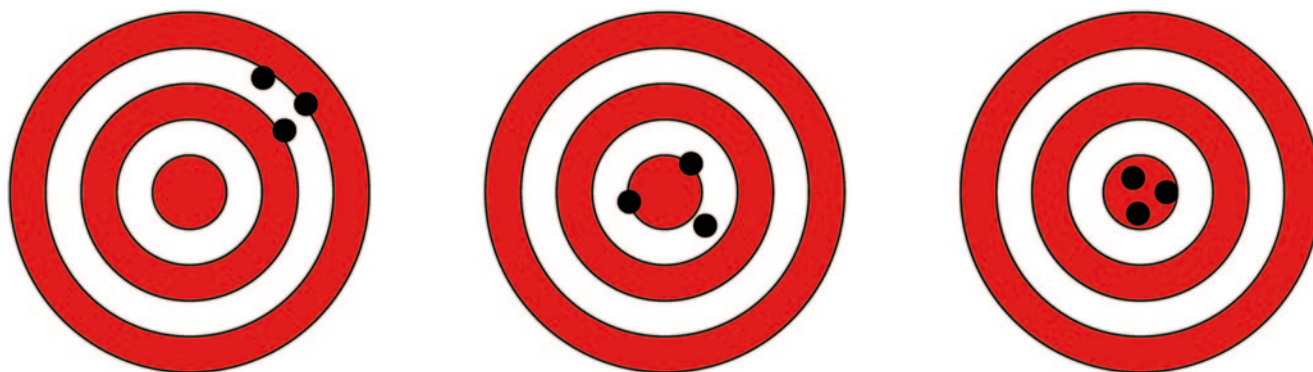
Fig. 5.7 Accuracy and precision. Left is precise but inaccurate; center is accurate but imprecise; and right is both precise and accurate
