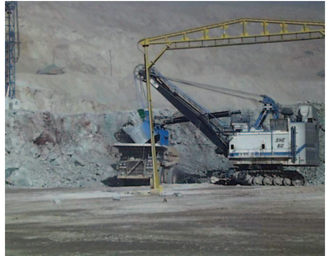
Fig. 7.1 Bucyrus SME 60 Shovel used at the large tonnage Escondida Cu Mine, Northern Chile (photo courtesy of BHP Billiton). Benches are 15 m high
