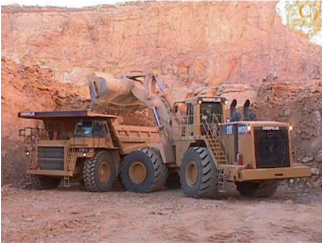
Fig. 7.2 Caterpillar 992 front-end loader used at Cerro Vanguardia's Osvaldo Diez vein. Cerro Vanguardia is a Gold-Silver deposit located in the Patagonia Region of Southern Argentina (photo courtesy of Cerro Vanguardia S.A.). Benches are 5 m high
