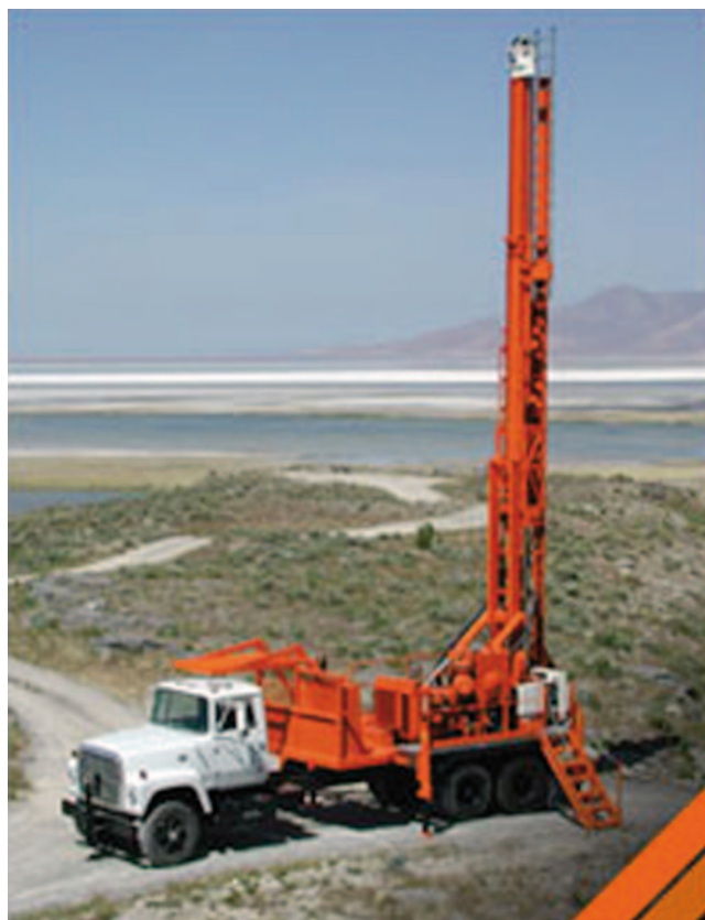
Fig. 5.1 Boart Longyear's LF-140-2 Core Drill Rig (diamond drilling)
