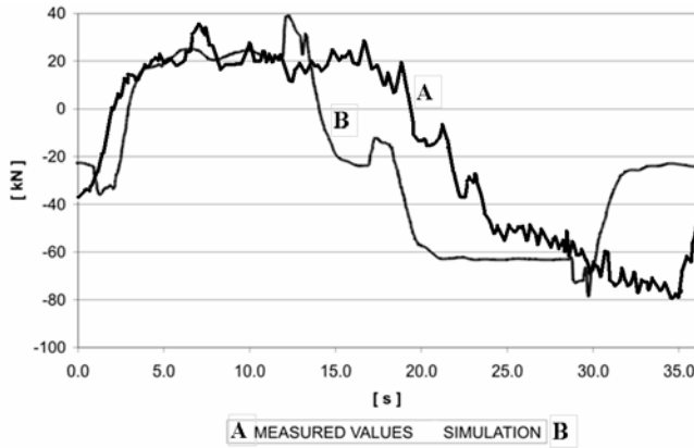
Fig. 11. The axial force of the right lower side brace during taxiing (“eight” manoeuvre).
