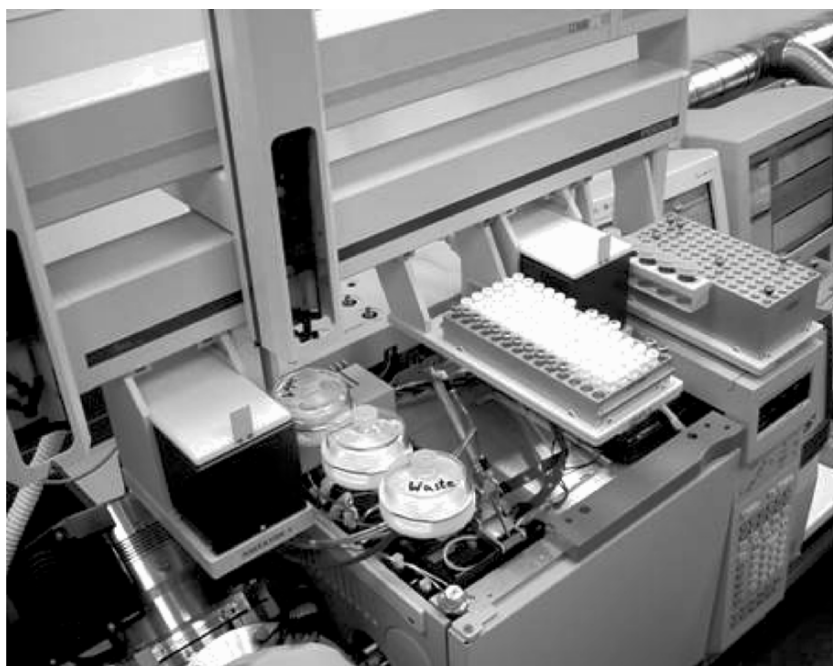
Figure 1-1. Image of a robotic system for sample derivatization, liner exchange, and gas chromatography/time-of-flight mass spectrometry (GC-TOF).
