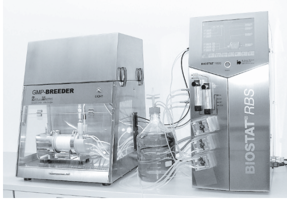
Figure 1. [BIOSTAT Bplus-RBS bioreactor with magnetic drive, operated in a GMP Breeder (Zellwerk), controlled by a BIOSTAT® Bplus unit (SBBI)].
