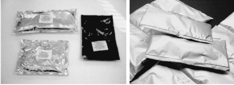
Figure 114. Macro encapsulation in bags (left from Climator/Sweden; right from Dörken/Germany)
