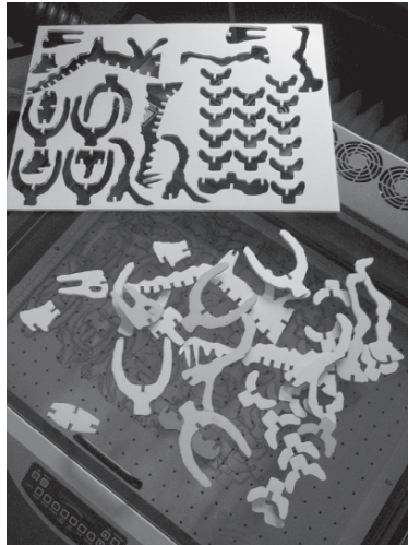
Figure 15. Physical dinosaur parts: The foam core sheet from which the pieces are cut sitting on top of the laser cutter. Below, unassembled dinosaur bones.
