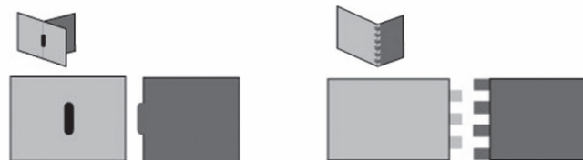
Figure 8. Connection conditions and joint types: Where a face and an edge connect, Furniture Factory creates a mortise and tenon joint. Where two edges connect in a corner the program creates a finger joint.
