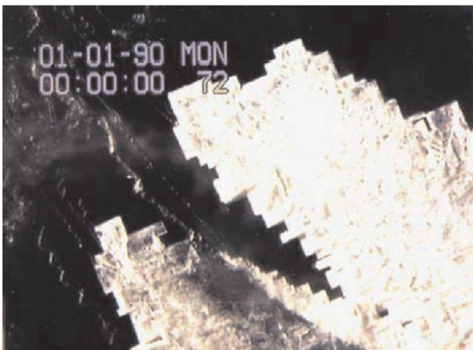
Figure 3. Thenardite ( \text{Na}_2\text{SO}_4 ) crystals grown on the coating of PAA-VLMW on calcite.
