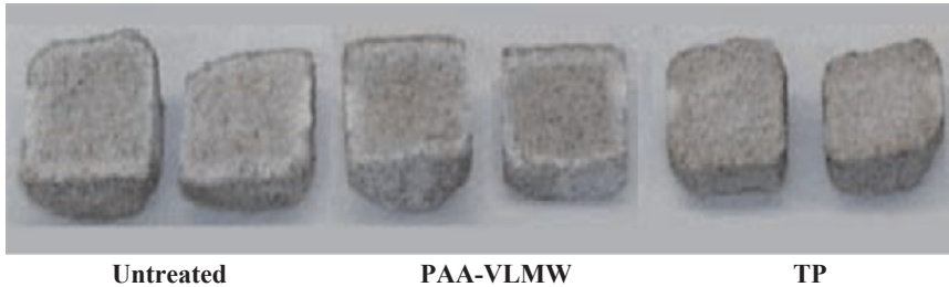
Figure 9. Salt distribution in samples split open after cycle 16 in Series 2. Efflorescence appeared after 10-15 minutes, indicating location of salt. Untreated stone and sample treated with PAA-VLMW has ring of salt within ~1 mm of surface, whereas all salt has retreated to the center of the sample treated with the terpolymer.
