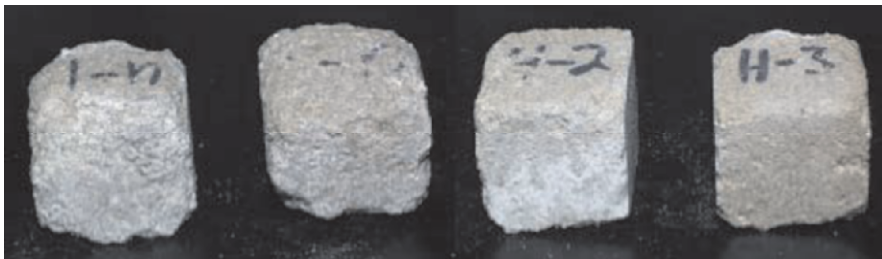
Figure 8. Trial 2 Cycle 16: Untreated stones (left two) and stones treated with PAA-VLMW (right two). Untreated stones begin to round off while the treated stones show only slight deterioration at corners and edges.
