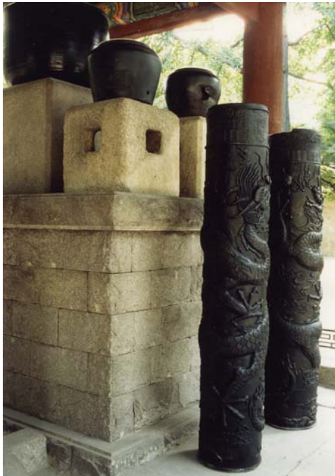
Time in Korea. Fig. 4 Relics of the self-striking clepsydra made in 1536 after that commissioned under King Sejong in the 1430s (Fig. 2). Shown here, from the upper left, are the reservoir for supplying water, compensator, and regulator vessels, and the two measuring vessels on the floor bed stand two meters high. The parts which announced time have been dismantled. (Korean National Treasure Number 229, the Jagyeongnu of the Borugak , preserved at the Deoksu Palace since 1938).
