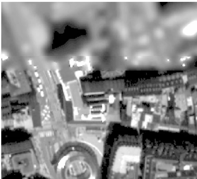
Fig. 11.3 Low resolution image with a high-resolution encrusted imagette with smoothed inner periphery
