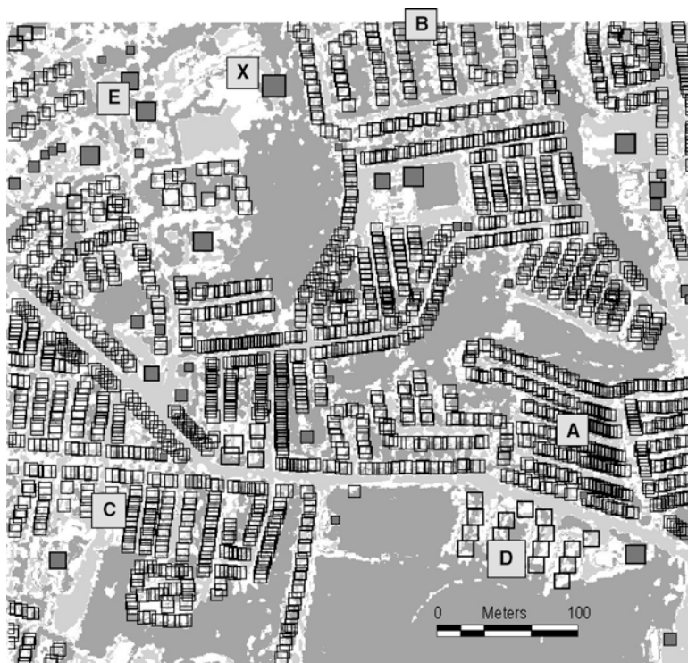
Fig. 8.6 Classified IKONOS image of Belfast subset: white areas represent pixels classified as residential, dark gray areas classified as non-built, and light gray as roads. Residential ( open squares ) and commercial ( shaded squares ) buildings from the COMPAS™ dataset are represented in proportion with area attributes. Note the very high density, linear arrangement of residential buildings at A; lower density, curvi-linear distribution at B; medium density, linear arrangement at C; and very low density, more uniform configuration at D. Only one commercial pattern is observable at E; and a school to the west of X
