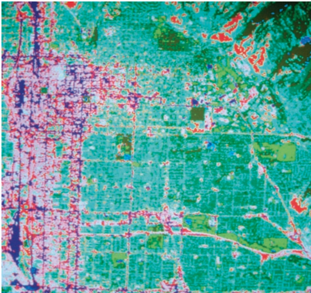
Fig. 6.11 V-I-S classified image/map of Salt Lake City and environs, according to the color scheme represented in Fig. 6.10. Overall, the image is a quite faithful representation of the urban/peri-urban environment (Chung 1989)
