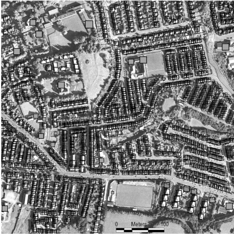
Fig. 8.5 Spatial correspondence between Cities Revealed™ aerial photograph of Belfast (at spatial resolution of 15 cm) and COMPAS™ points (squares proportioned by area attributes)
