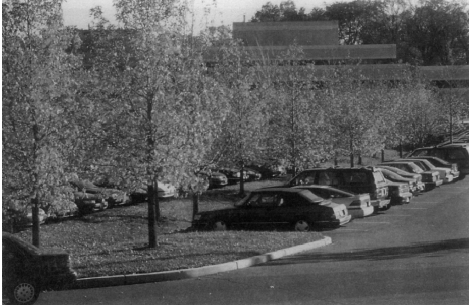
FIGURE 12. The island in this corporate parking lot provides an opportunity for significant tree plantings as well as storm water detention and infiltration.
