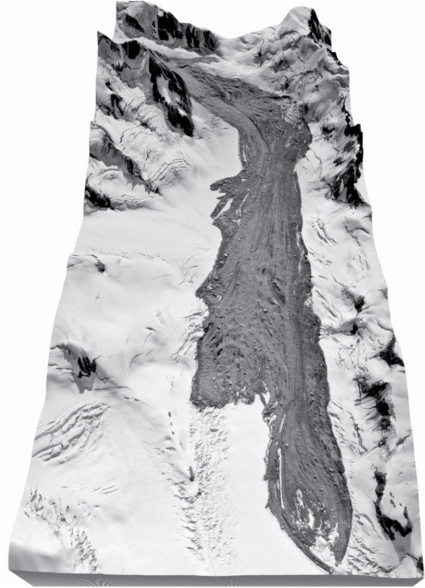
Figure 9. Perspective view to the southeast of the 1997 Mount Munday rock avalanche on Ice Valley Glacier, Waddington Range, southern Coast Mountains. This digital image was prepared from aerial photographs flown on August 20, 1997, and consists of a DEM with an orthophoto drape. Note flow lines in the debris. Elevation of the top of the source area is 3000 m.a.s.l. and the lower tip of the debris is at 2100 m.a.s.l. The length of the rock avalanche path is 4.7 km [95].
