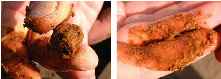
Figure A24 Thixotropy. Undisturbed clod is shown on to the left, but disturbed clod to the right. The soil reaches the liquid limit when disturbed with gentle pressure, even though the clod appears relatively dry. The soil is hydric andosol from the Azores (Portugal).
