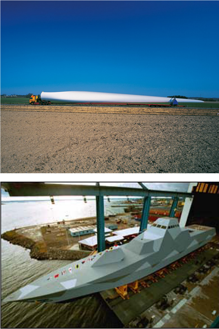
Figure 1.2 Examples of sandwich structures.
