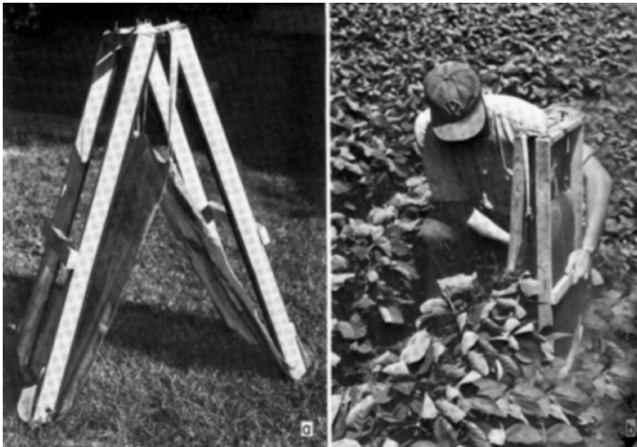
Figure 6.8 (a) a clam trap used for sampling arthropods from a 30 cm segment of a row crop such as soybean; (b) use of clam trap in a soybean field (Source: Mayse et al. , 1978) Reproduced by permission of The Entomological Society of Canada.
