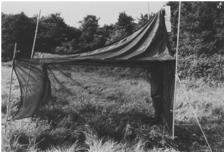
Figure 6.9 A Malaise trap of the type manufactured by Marris House Nets, UK.
