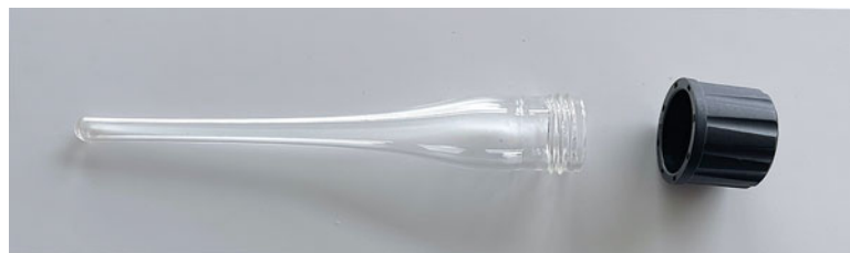
Fig. 2 New tubes for Multivapor manufactured by ALAMO (Madrid, Spain)
