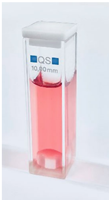
Fig. 1 4-Way clear 1-cm path length quartz fluorescence cuvette used for analysis of diluted red wine samples
