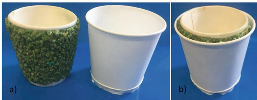
Fig. 1 Packaging functionalization: (a) Particles distributed onto the external surface of the cup and the cup without bottom; (b) final packaging
