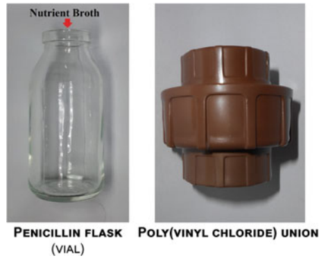
Fig. 1 Materials for the determination of microbial permeation
