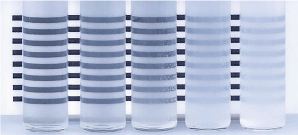
Fig. 1 McFarland standards representing different microbial concentrations (left to right: 0.5, 1.0, 2.0, 3.0, and 4.0 McFarland unit), positioned in front of a Wickerham card. (Adapted from Bioanalytic GmbH [ www.bioanalytic.de ] with permission)
