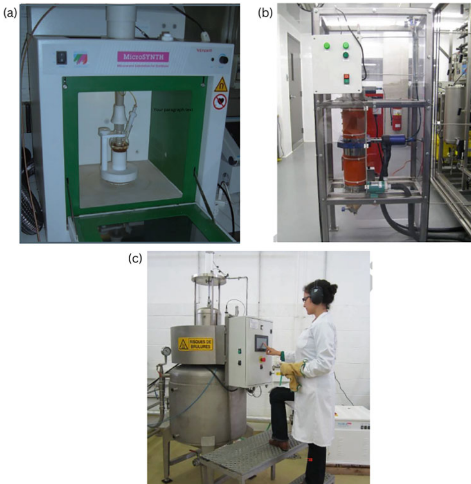
Fig. 3 Hybrid extraction techniques (a) ultrasound-microwave extraction, (b) ultrasound-supercritical fluid extraction, and (c) ultrasound-DIC extraction. (Reproduced from Chemat et al. [4] with permission from Elsevier)
