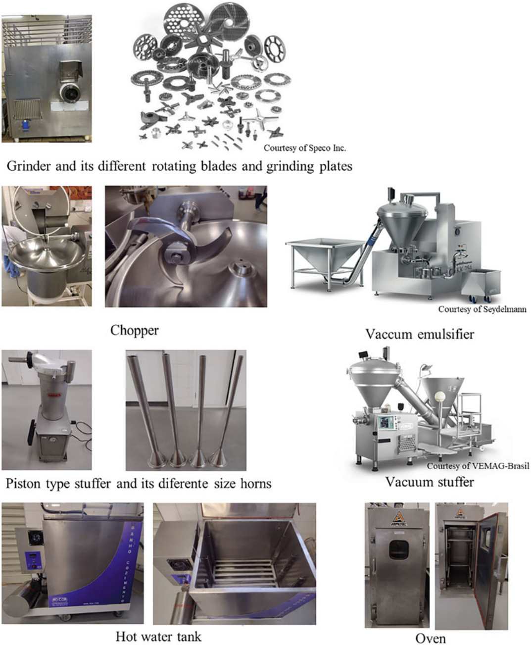
Fig. 2 Equipment used in the processing of emulsified meat products. (Photos by Paglarini (Meat Laboratory of School of Food Engineering, State University of Campinas))
