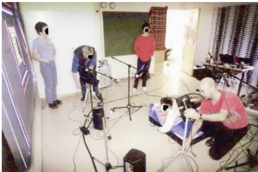
Fig. 7.4 A three-sensor set-up using infrared sensing with volumetric profiles with participant on vibroacoustic chamber generating motion data that results in sounds and coloured images on a large projection screen in front of her
