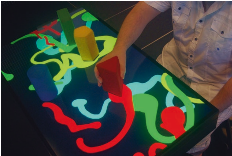
Fig. 2.2 An individual using the EDNA system explores the functions of several soft graspable tangible user interfaces to draw and paint digitally
