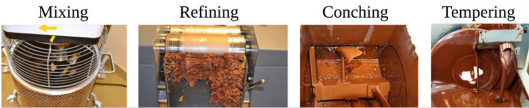
Fig. 2 Chocolate processing during mixing, refining, conching and tempering steps. (Adapted from [31, 32])
