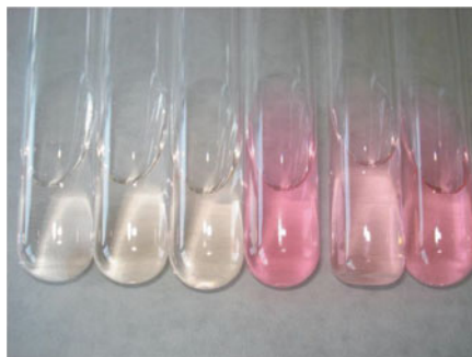
Fig. 1 The reaction between malonaldehyde (MDA) and thiobarbituric acid (TBA) forms a colored adduct
