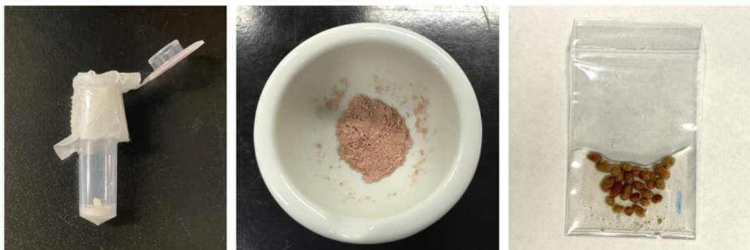
Fig. 1 Sample preparations for BA analysis. (a) Blood plasma was subjected to lyophilization in a tube covered with paper. (b) Lyophilized rat liver was ground with a pestle and mortar. (c) Fecal samples were soaked in water for a day and were then ground before freezing
