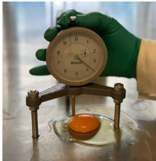
Fig. 3 Measuring Haugh units from dense albumen
