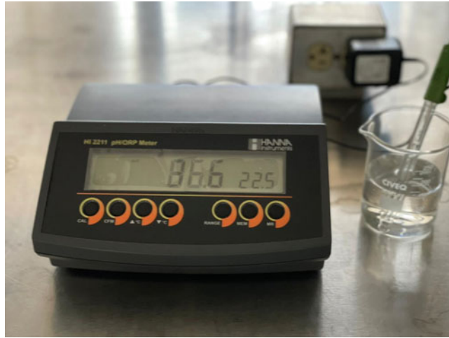
Fig. 2 pH/ORP meter to evaluate electrolyzed water
