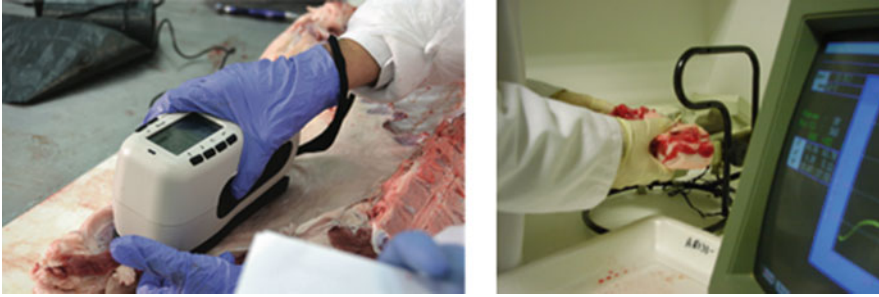
Fig. 4 Color coordinates L^* , a^* , and b^* assessment by a Minolta chromameter
