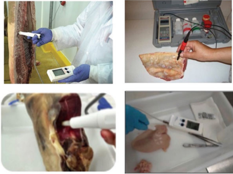
Fig. 3 pH measurement in a carcass, a piece of meat, and a processed meat product
