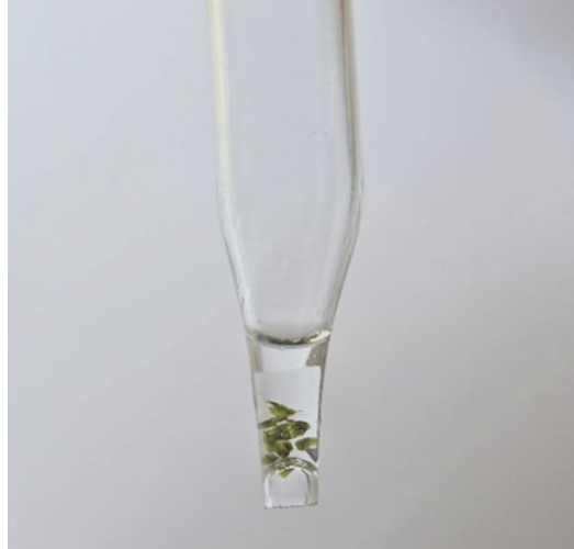
Fig. 6 Ten potato shoot tips contained in a small volume of PVS2 in the tip of a Pasteur pipette, before it is placed on the aluminum foil strip
