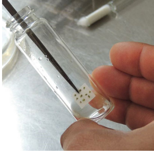
Fig. 4 A piece of filter paper (1 × 1 cm) with 10 potato shoot tips is introduced to a screw-top glass tube (70 × 20 mm), containing ~1.0 mL of loading solution (LS). Shoot tips are treated for 20 min with LS (at room temperature). After 20 min, LS is replaced with ~1.0 mL of ice-cooled plant vitrification solution 2 (PVS2)
