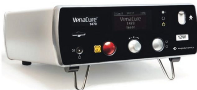
Fig. 34.7 VenaCure 1470 nm laser device (AngioDynamics, Latham, NY)
