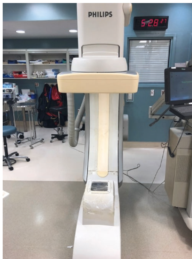
Fig. 19.1 X-ray generator and image intensifier
