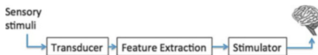
Brain-Machine Interface: Overview, Fig. 1 Basic elements of an afferent BMI. Features are extracted from the sensory stimuli and then converted to electrical pulses that
