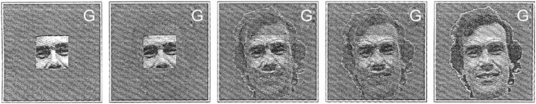
Synergetics: Basic Concepts, Fig. 6 Pattern recognition by the synergetic computer: recognition of a specific face of which initially only a subset of pixels is presented (Haken 2004a)
