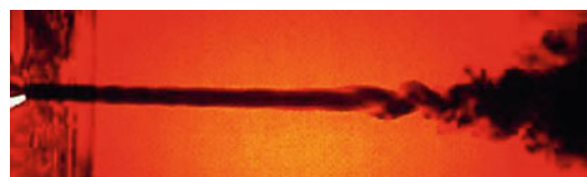
Fluid Dynamics: Turbulence, Fig. 1 Development of turbulent structures in a free jet experiment
