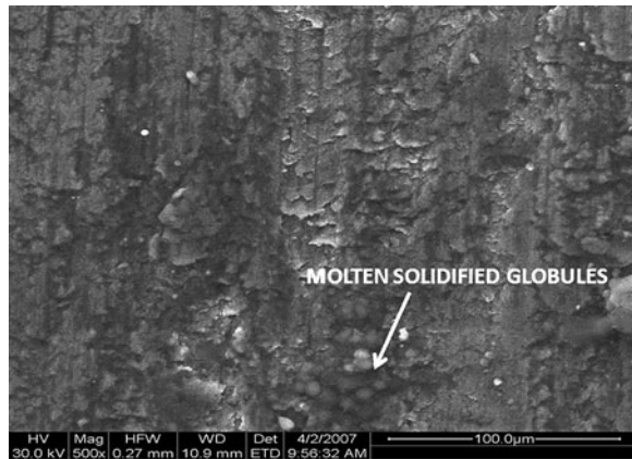
Fig. 5.23 Ground surface texture for grinding condition V = 1,400 m/min, s = 0.6 m/min, a = 20 \mu\text{m} [SiC wheel]
