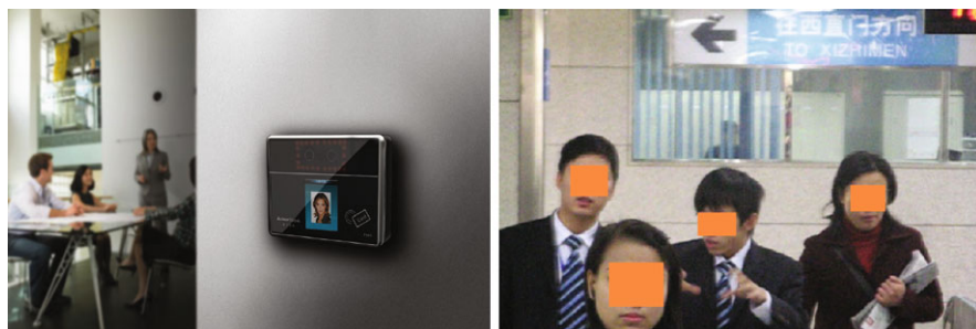
Fig. 1.9 An embedded NIR face recognition system for access control in 1:N identification mode and watch-list face surveillance and identification at subways
