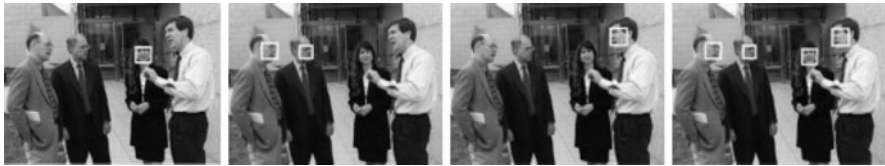
Fig. 11.12 Merging from different channels. From left to right: Outputs of frontal, left, and right view channels and the final result after the merge
