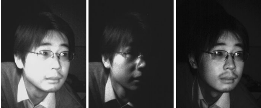
Fig. 15.3 From left to right: a Face image in mixture of sunlight and active NIR light; b face image in sunlight only, c image difference (a)–(b)
