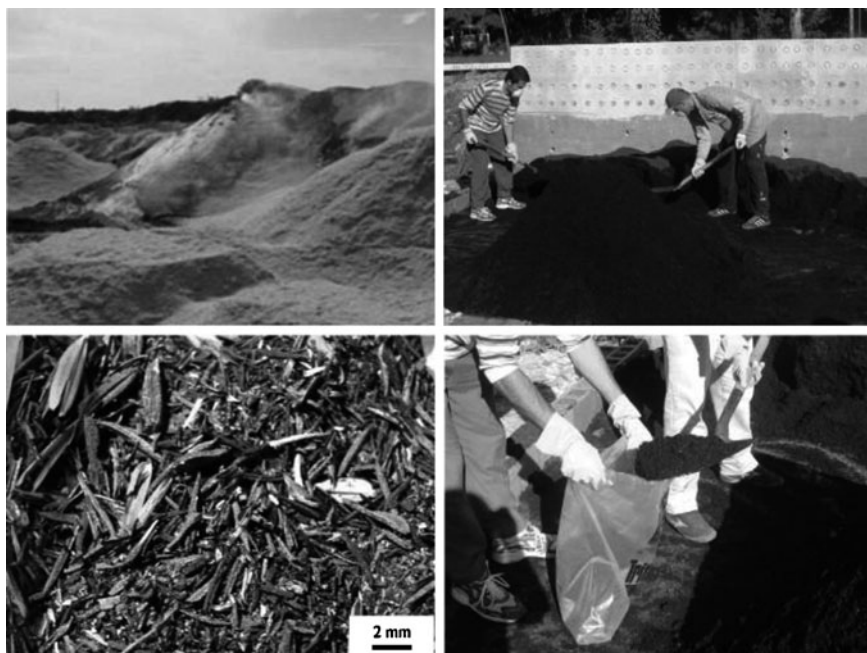
Fig. 5.3 Natural rice husk ashes produced in Brazil. Left open field burning and aspect of the ashes; right storage and homogenization processes for laboratory studies (Zerbino et al. 2011)
