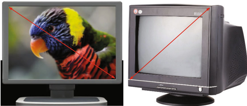
Figure 26.2: LCD and CRT Diagonal Sizes.
