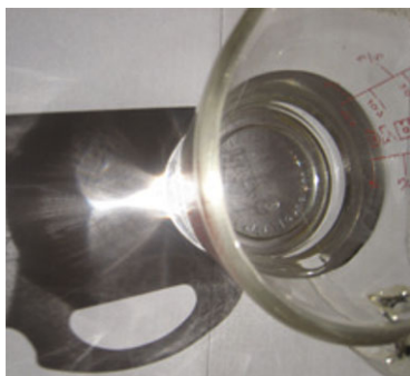
Figure 17.17: Caustic Cast by Water in a Glass.
