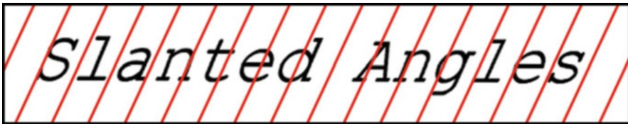
Fig. 8.21 Slant projection lines using angle obtained from Fig. 8.20
