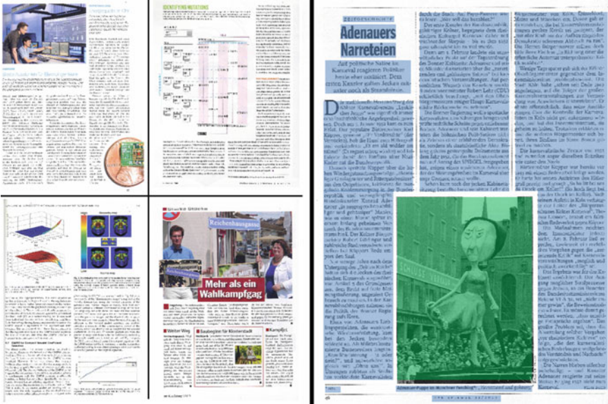
Fig. 30.6 Sample pages for layout analysis on the left and an example for a ground-truth layout analysis of a magazine page on the right. (These types of pages are used in [3] for layout analysis performance evaluation.)
