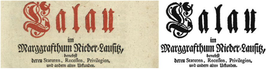
Fig. 30.4 Image of a part of a book page, left side color image, right side corresponding binary ground-truth (GT) image
