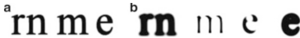
Fig. 2.15 (a) Original characters and (b) characters after degradation. Through touching and broken artifacts, recognition algorithms can easily misclassify the characters
