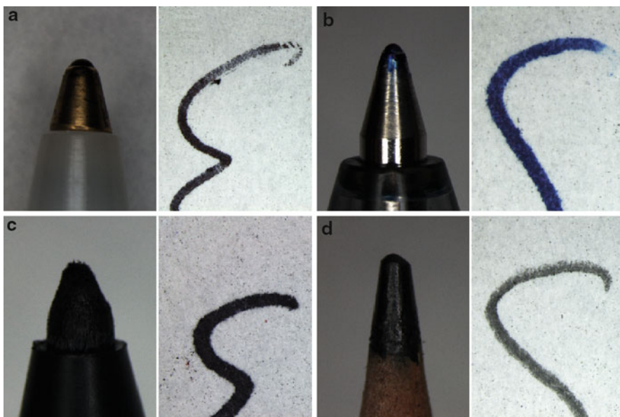
Fig. 2.3 Examples of writing tips and writing samples for (a) ball point, (b) gel (c) felt tip and (d) pencil
