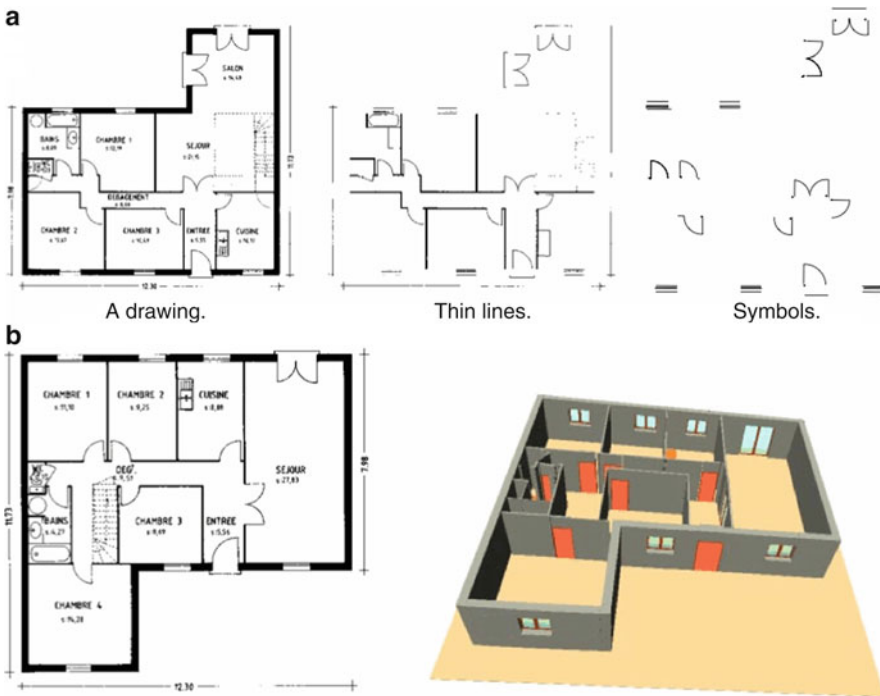
Fig. 17.6 Taken from [15] representing the results at all major bottom-up stages of the interpretation process: line segmentation, symbol recognition, context identification, 3D reconstruction
