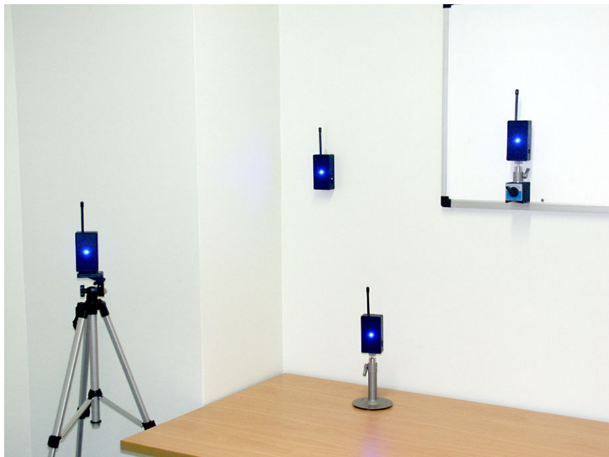
Fig. 7.2 Point targets implemented using ultra bright LEDs
