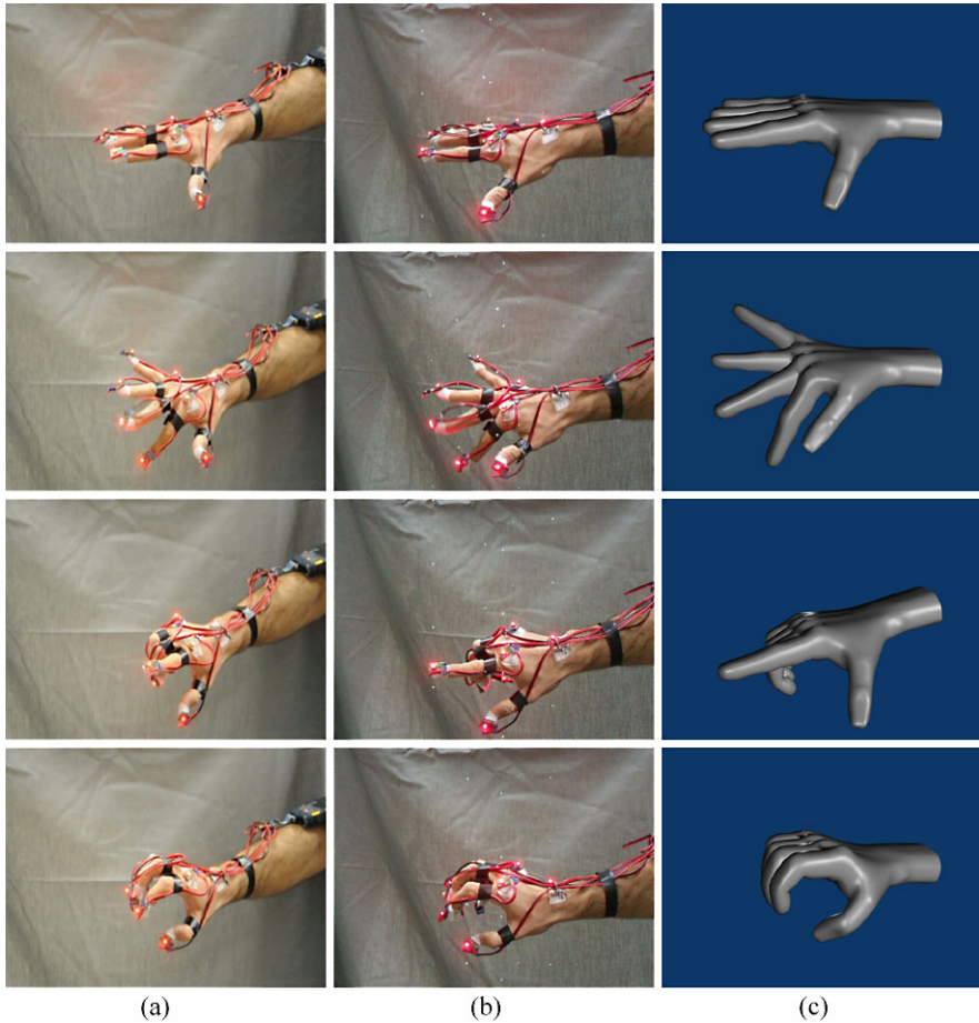
Fig. 3.7 An example of hand reconstruction using our methodology at a frame rate of 100 Hz. (a) View of the hand from RGB camera 1, (b) a different view of the hand from RGB camera 2 and (c) the final visualised posture. The resulting poses are visually natural and biomechanically correct
