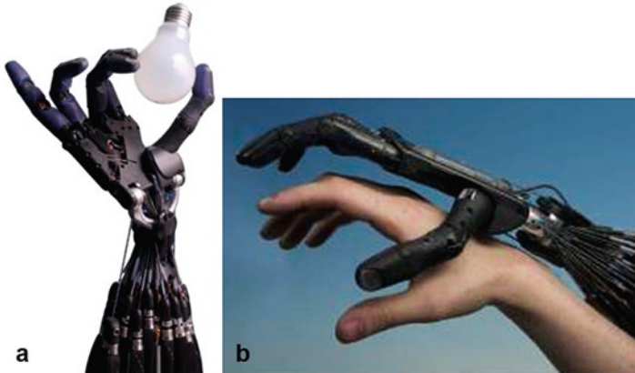
Fig. 4.2 The Shadow Dexterous Hand ( http://www.shadowrobot.com/hand/ ) has been designed to have a range of movement (approaching) equivalence to that of a typical human being (27 DOF) with 20 degrees of freedom
